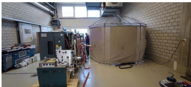
Figure 4. Experimental setup by PSI and FORTH for dynamometer emission measurements in the BFH facility.
