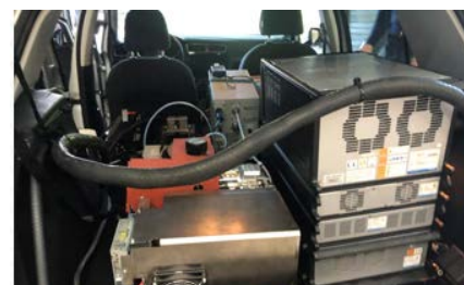
Figure 3. FTIR Exhaust Gas Analyzer device, Horiba FTX-ONE-CS (modified for on road measurement) and PEMS installed in a car.
